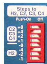
Figure 9: Temperature steps to cooling stages C2 and C3, and to heating stage H2.
