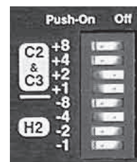
Figure 9: Temperature steps to cooling stages C2 and C3, and to heating stage H2.
