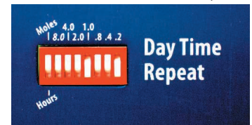
Figure 2: Day Time Repeat interval set to trigger irrigation cycle after 1.2 Moles of accumulation of sunlight. 1.2Moles equals 120 changes of the Solar Count LED or 60 on-off cycles.
