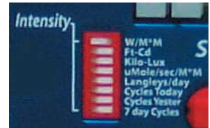
Figure 6: Display of solar intensity or number of recent cycles is controlled by switch shown below.
